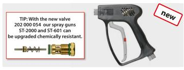
Professionel spray gun. Ceramic ball, chemical resistant valve and acid and alkali resistant PEEK sealing seat. FKM seals.
